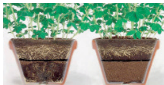
Bituminous Waterproofing membrane without and with antiroot additive Preventol B5 .
